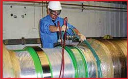
NB Finishing Company can utilize 33 years of expertise to follow the process of applying a homogenous bond to selectively repair specific non-conforming or damaged areas without removing the component part from the assembly. The end result is a component part that meets or exceeds the performance and durability of the original OEM manufacturer part.
